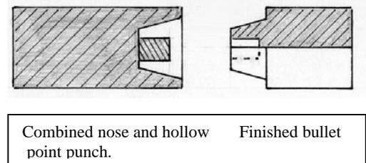
The shape of the hollow point is usually round but it can be made square, hexagon, star shaped, or just about anything else. Since the cavity is formed by a punch the punch can be machined to produce about any cavity shape wanted.
