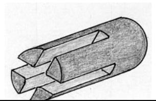
Slotted core and finished Keith type bullet. Slots close up leaving only faint lines on the bullet.
