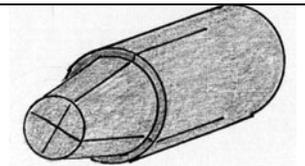
On impact the slots, if deep enough, will cause the bullet to break into four pieces or if the slots are shallow will cause the bullet to mushroom quickly.
