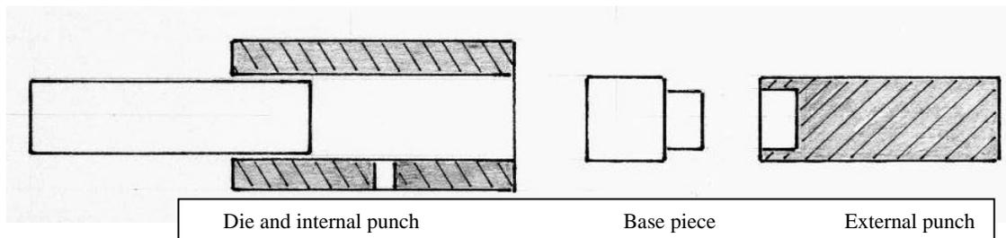
When all of the base pieces are made, they are set aside and the nose pieces are made. The bullet can be a semi-wadcutter type or a smooth ogive type. For handgun or plinker loads the SWC type of bullet works well. But for serious hunting and target bullets the smooth ogive bullet is better. The smooth ogive type of bullet is shown here.
