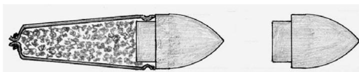
Sectioned paper cartridge and heel base bullet
