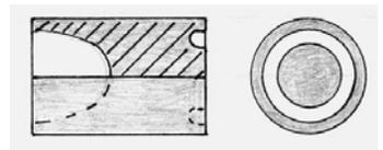
It is commonly thought that the hollow base makes for a more accurate bullet by making the bullet nose heavy like a badminton birdie or shuttlecock. In fact the hollow base design is one of the worst for accuracy except when the range is close and light powder charges are used.
