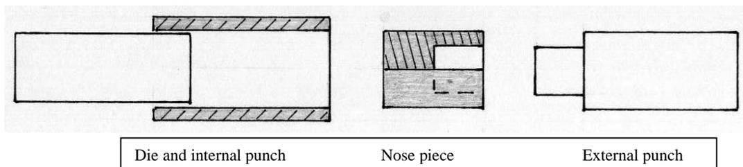
The core seat die is removed from the press and a point form die is placed in the press ram. The point form die is slightly larger than the core seat die so that the nose piece will easily fit into the die. Because of this the external punch is replaced with a little larger punch with a tang on it. The nose piece is placed in the die, swaged, and ejected from the die. The nose piece now looks like a bullet that has a straight, hollow cavity in its base.
