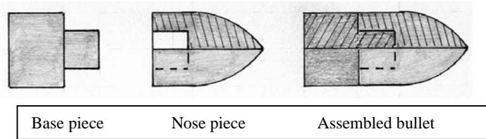
The idea is simple enough, part of the bullet is made from soft lead and part is made from harder lead. The two pieces are assembled and swaged together.
