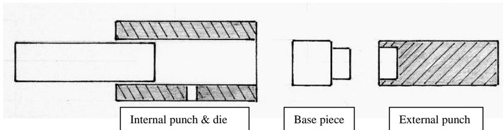
Once the base pieces are made they are set aside and a preform for the nose piece is made. The core forming die is again used to make the preform, however, the external punch with the cavity in it is replaced with a hollow cavity forming punch. The preform is now a flat ended cylinder with a hollow cavity.
