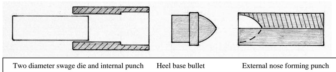
The one problem with this type of setup is that the length of the heel cannot be changed. This is usually not a problem unless the bullet maker wants to experiment with different lengths, or bullets are to be made for different cartridges that require various heel lengths.
