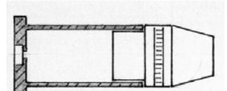
Cartridge loaded with a heel base bullet. The cannellure outside of the ctg. case held lube.
