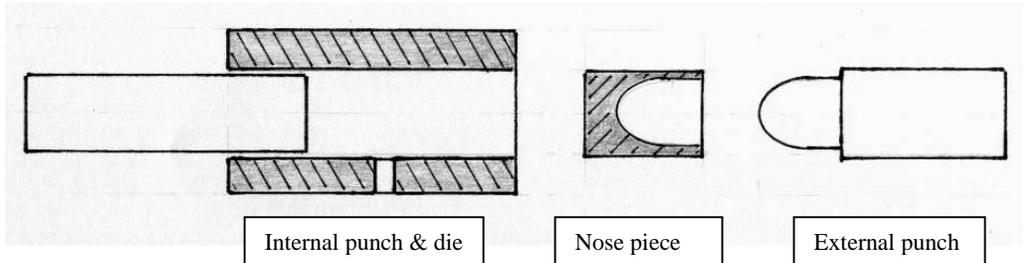
This is now placed into a point forming die and the preform is given a bullet shape. Both the base piece and the nose piece are cleaned with acetone and dried. The nose piece is filled with talcum powder leaving room for the base piece to be pressed in.
