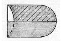
**A bevel base** bullet is sometimes used when loading quantities of ammunition with a progressive loading machine. The bevel helps to start the bullet into the cartridge case and reduces the chance of “shaving” the bullet. It is a useful design when loading a lot of ammo in a hurry.
