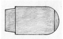
The rebated boattail (RBT) is made by using a punch that has the RBT shape machined into it. This punch may be the internal punch in the case of a SWC die or it would be the external punch if a point forming die is used to make a smooth ogive bullet.
