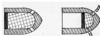
Unfired bullet on the left. Fired bullet on the right with lube extruded through holes in the bullet's ogive.
