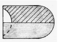
A cup base is sometimes used with pistol bullets or shotgun slugs to move the weight of the bullet forward a little. This can easily be overdone so that the bullet is unstable in flight but it can be helpful sometimes.
