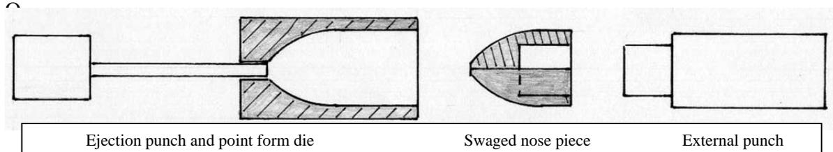
Once all of the nose and base pieces are formed the parts are cleaned with acetone, MEK, or other solvent to remove any lube on the parts. It is sometimes necessary to lightly roughen the tang on the part using a side cutter or pliers to insure the two pieces stay together after the final swaging, but usually this isn't needed.
