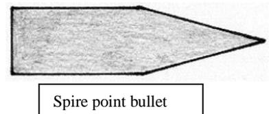
Both the spire point and the secant ogive have an abrupt change where the ogive and bearing meet but there is no step or shoulder. The secant ogive is often used when making VLD (very low drag) type bullets. It permits the use of a very sharp point on the bullet while keeping the ogive length within reason. It is a useful design but mostly seen in long range metal jacketed target bullet or some military bullets.
