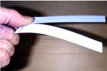
Testing for grain direction
