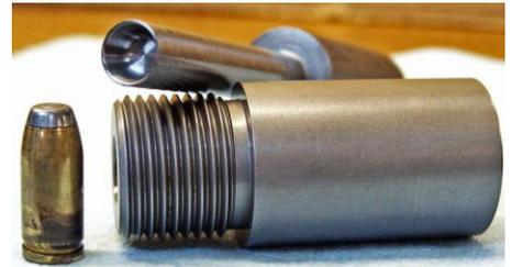
Lead tip die and internal punch. The cavity in the punch reshapes the soft point on the bullet.
