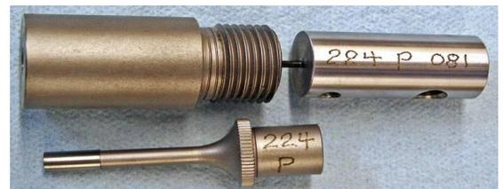
Point form die & punches. The die and punches are marked with the bullet *diameter*, the letter P for point form, and the ejection punch is also marked with the ejection pin diameter.
